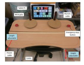
Fig. 4. (Color online) Wrist rehabilitation mechanism.
